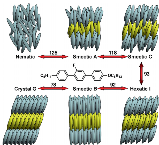
Figure 5. The change in the structures of the liquid crystal phases formed when the laterally fluoro-substituted terphenyl is cooled from the isotropic liquid or heated from the anisotropic plastic crystal G phase.
